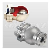
Ayvaz SK-61 float <u>steam traps</u> especially perform continual evacuation at the steam saturation temperature. Ayvaz SK-61 doesn't affect instantaneous and large pressure shift. SK-61 is mainly applied at the systems where the condensate is evacuated rapidly and it is also ideal for automatic temperature control system.
